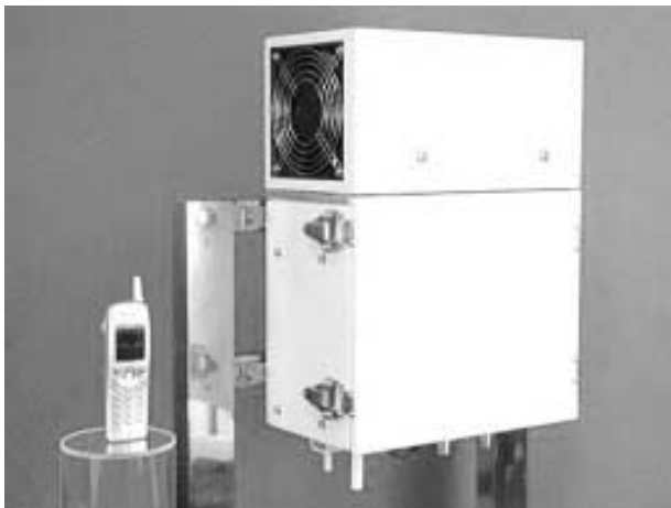
図-7 超伝導フィルタ搭載の屋外受信増幅装置の試作機 Fig.7- Developed open-air receiving front-end with HTS filters for 2 GHz band.
