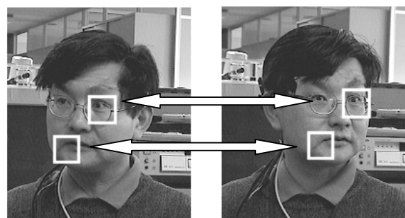
図-15 局所パターン照合法 Fig.15-Local feature-based matching.
