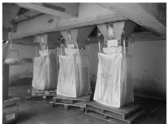
図-5 酸化銅の回収工程 Fig.5-Process of collecting copper oxide.
