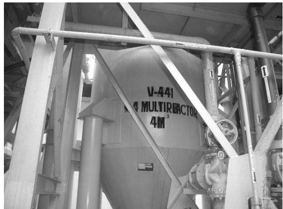
図-4 酸化銅処理設備の酸化反応槽 Fig.4-Reactor of treatment copper oxide.
